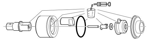
Spread a layer of grease on all sliding and impact surfaces. Use the rest of the grease, approximately half the amount, inside the cavity of the hammer and on the driver flange. Total grease amount **8.5**ml.
