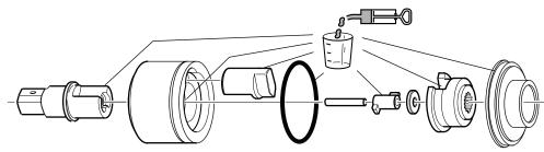
Spread a layer of grease on all sliding and impact surfaces. Use the rest of the grease, approximately half the amount, inside the cavity of the hammer and on the driver flange. Total grease amount 21ml.
