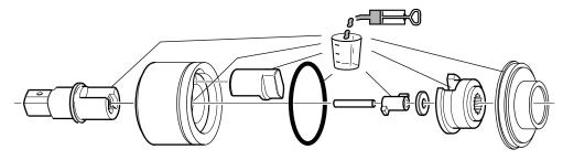
Spread a layer of grease on all sliding and impact surfaces. Use the rest of the grease, approximately half the amount, inside the cavity of the hammer and on the driver flange. Total grease amount 7ml.
