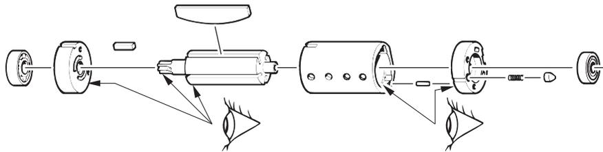
Assembly - according to Bäckströms method
